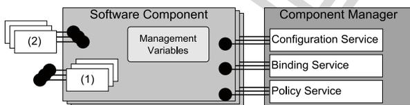
Figure 1: Component Structure
